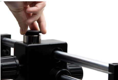
Fig. 9—(Right) Reinstall the cap in the top of the post and screw it clockwise to tighten it.
