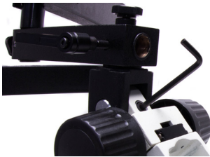
Fig. 20—Adjust the tension on the focus mount hinge using the hex key provided with the 502009 focus mount.
